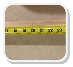
Use the measuring tape and pencil to mark the wide faces of the 72-inch boards, 20-inches from the end.
